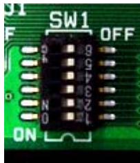
Figure 2 Switch for Masking Signals
